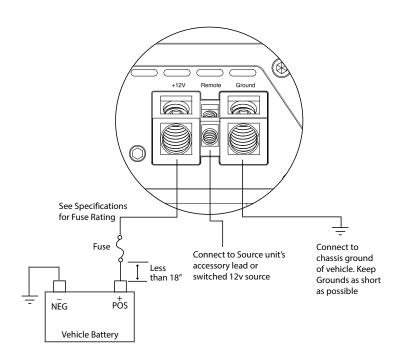
For maximum current flow, Aunex recommends that you tin your ground wire before connecting it to the ground terminal of your amplifier. In addition, Aunex recommends using high quality 100% OFC (Oxygen Free Copper) or Tinned 100% OFC speaker wire. This will ensure that your speaker / subwoofer receives maximum output from your amplifier.
