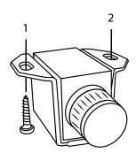
17. Phase Switch (AE1800.5D Only): Depending on the absolute phase of your main speakers and amplifier and the distances of the subwoofer and the main speaker from the main listening position, the bass in the crossover region maybe smoother if you reverse the subwoofer's phase. Try both settings to determine which polarity produces the best overall bass performance in your system. Typically, though, phase is left at the 0° for most installation.
